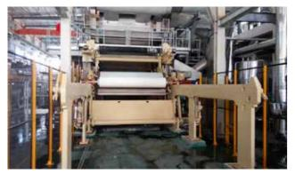
increase the company's tissue production by 42,000 t/y. Toscotec's scope of supply includes a MODULO-PLUS *ES* machine, designed for a speed of 1500 m/min, featuring TT SYD-15FT (4572mm) and double press configuration, Milltech's steam-heated hood, stock preparation equipment, electrical and control systems, spare parts for the entire plant and a full service package.
