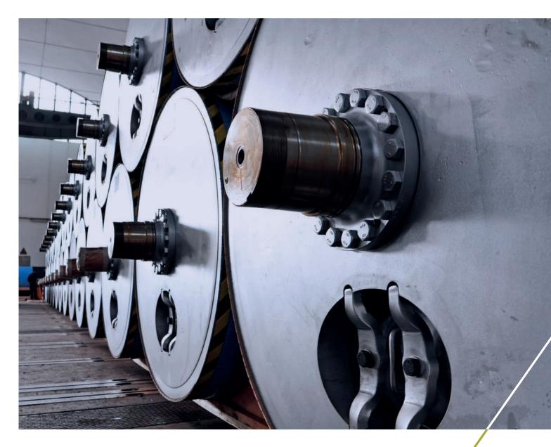
the rebuilding is to implement machine efficiency, reliability and safety in operations. Toscotec's delivery includes 25 new TT SteelDryers in place of casted iron dryers, that will allow the paper mill to increase its drying capacity, production and the width of the paper produced. The existing mechanical drive will be replaced with a new silent drive system. Tail threading will be ropeless from the press section through the new dryer section up to the pope reel.
